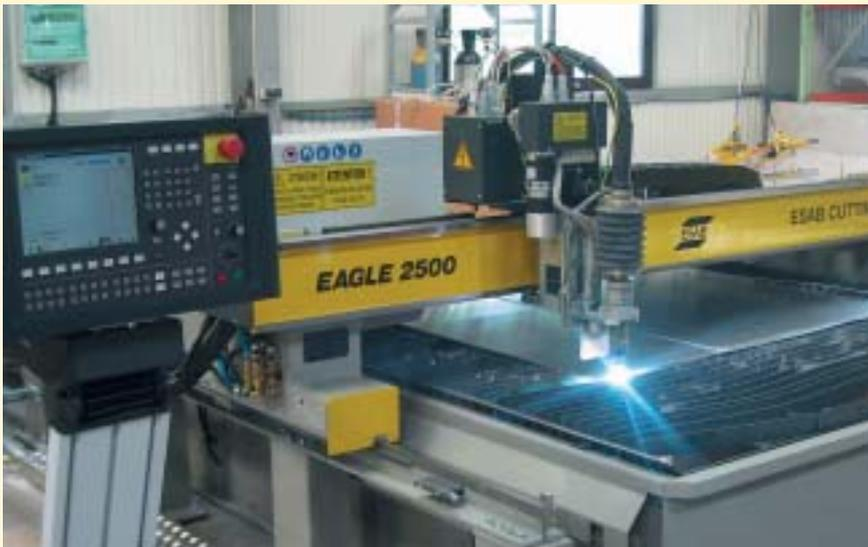
A latest range of plasma cutting machines from ESAB uses new production technologies to improve material utilization and increase plate handling efficiencies.
