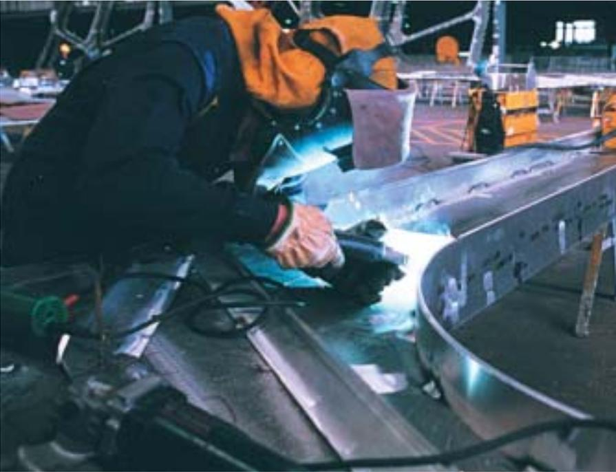
*Figure 2. GMAW being used on high strength large aluminium structural components at Incat's Shipyard in Australia*
