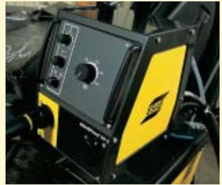
er is to be used as part of a semi-automated welding system, a remote control output provides a 42V AC power supply, start/stop control and remote monitoring and control of the welding current and voltage, depending on the power source employed.
