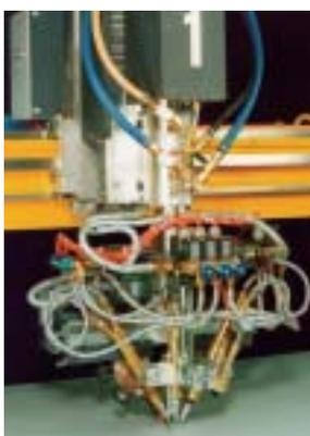
Figure 6. The endless rotating head allows bevelling to any shape.
