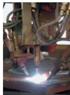
Figure 7. The tangential position of the head relative to the contour.
