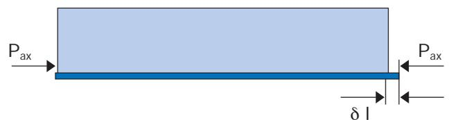
Figure 10. Elongation of flange during welding
