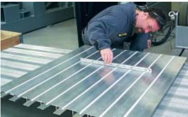
Figure 1. Friction stir welded, straight panels under inspection at ESAB FSW Center of Excellence in Sweden.
