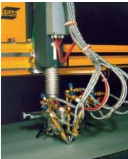
Figure 4. Manual bevelling head.
