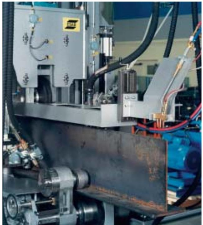
Figure 4. ESAB's T-beam welder IT258 with Propane torch heating/straightening.
