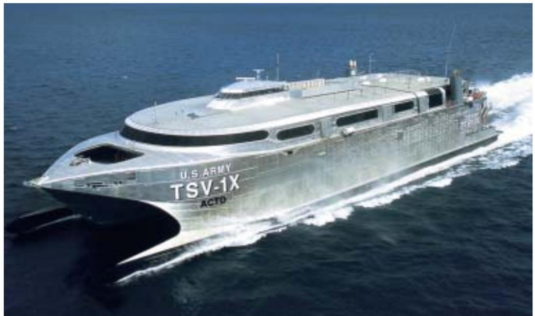
Figure 1. The Spearhead - new generation of 98-metre wavepiercers
