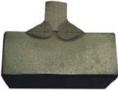
Figure 8. Cross section of welded T-beam.
