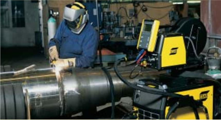
ESAB's new AristoMig Universal welding machines are suitable for welding virtually all weldable metals, ranging from mild steel to the most advanced nickel-based stainless steels and aluminium. As well as MIG/MAG and pulsed MIG, the units can also be used for DC-TIG, pulsed TIG and MMA welding, or for Carbon Arc gouging.
