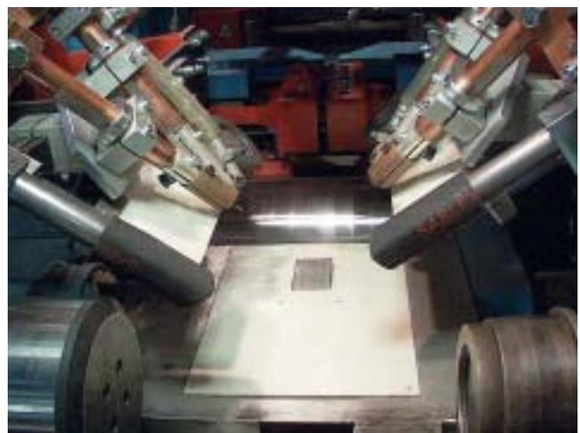
Figure 7. DC-AC Torch arrangement in ESAB's T-beam welder.
