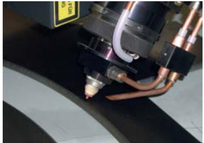
Figure 18. Bevelling capacity up to  $45^\circ$  on 10mm carbon steel and  $30^\circ$  on 12mm carbon steel.
