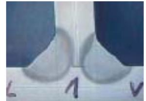
Figure 3. safe penetration in vertical down welding with OK Tubrod 14.12.
