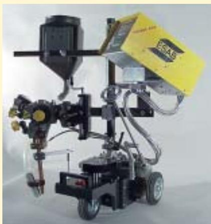
**A2 TRIPLETRAC, THREE-WHEELED SAW TRACTOR FOR PRECISION JOINT TRACKING**
