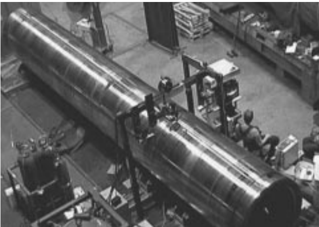
Figure 3. Welding tests running in the industrial environment. Base material welded was PM Duplok 27, with wall thickness 85 mm and outer diameter 1320 mm.
