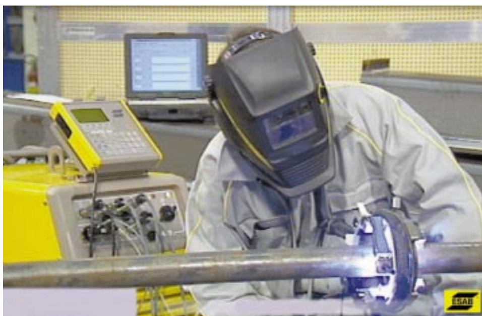
Figure 4. Quality assurance application for Protig 450, TIG welding tool PRC and PC computer.
