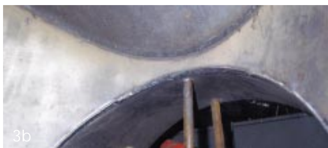
Figure 3: Waterbox welded with PZ6113-1.2.
