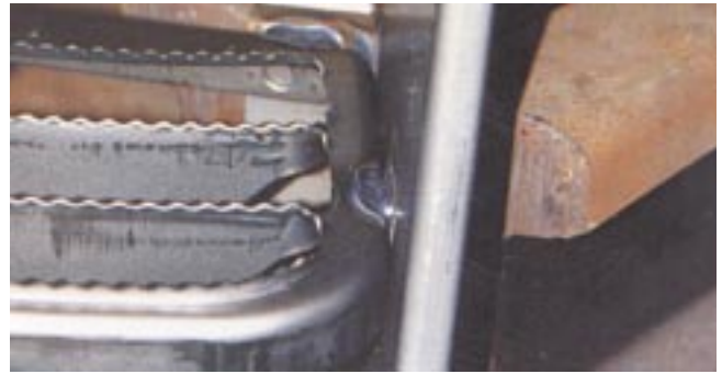
Figure 7: Attachment welds on vehicle stairs in 2 mm thick sheet metal. Spatter free welded with PZ6105R-1.4 mm.
