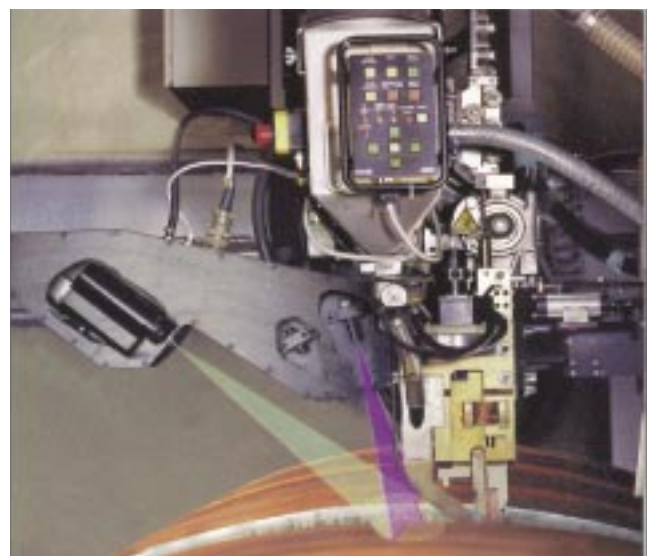
Figure 6. The ABW welding head and its smart camera and linear laser.
