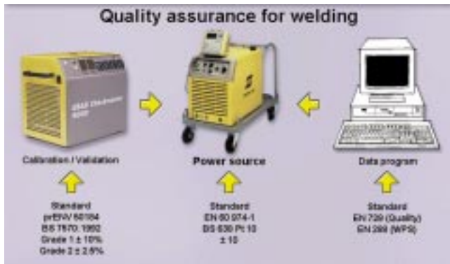
Figure 3. Power source validation and standard verification.
