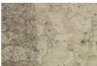
Fig. 9. Fusion line, weld metal on left. No grain growth seen at heat affected zone. Delta ferrite in weld metal is etched dark. Base metal TP 316 LNG and filler wire OK Autrod 16.32. Magnification 75 x.
