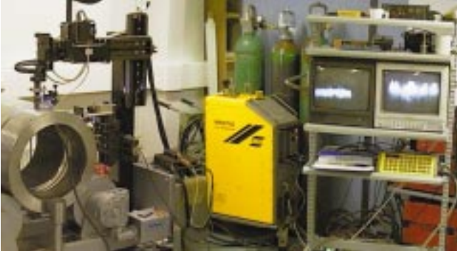
Figure 2. Welding test arrangement in the laboratory conditions. Base material welded was PM Duplok 27, with wall thickness 70 mm and outer diameter 600 mm.
