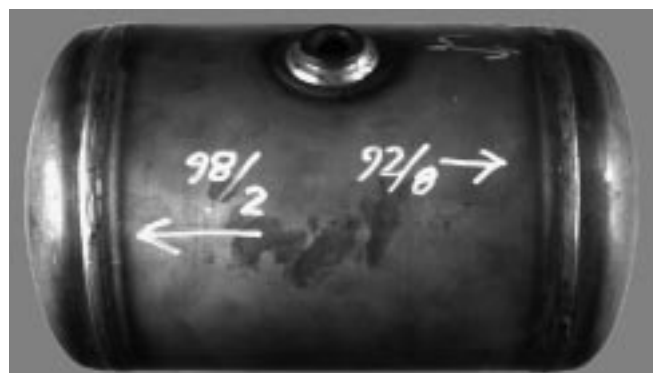
Figure 3: Boiler with two joggled circumferential joints, welded with PZ6105R-1.4 mm in 60s. Mechanised welding.
