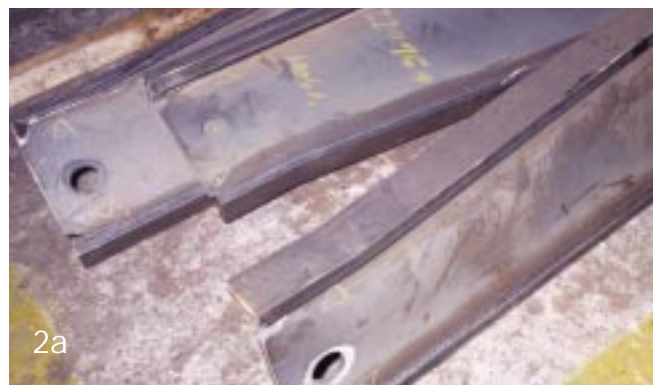
Figure 2: Welding of beams with PZ6113-1.2mm
