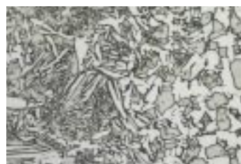
Fig. 11. Fusion line, weld metal on left. No grain growth or changes in phase balance can be seen at heat affected zone. Delta ferrite is etched dark. Base metal PM Duplok 27 and filler wire D27. Magnification 300 x.
